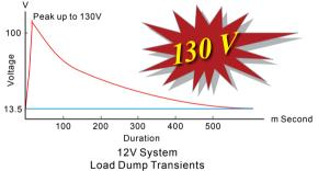
Load dump transients typically reach peak voltages of 130 volts in 12 volt systems with relatively slow rise times.
