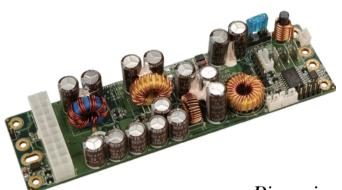
Dedicated ATX power for car PC and battery powered applications
